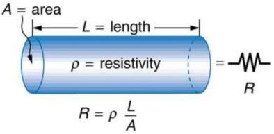
Q2: Will current flow more easily through a thick wire or a thin wire of the same material, when connected to the same source? Why?
